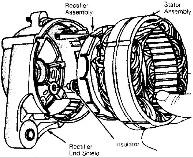
Fig. 9: Removing Rectifier & Stator Assembly Courtesy of Chrysler Motors.
