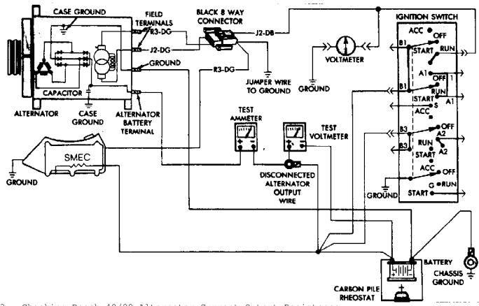
Fig. 3: Checking Bosch 40/90 Alternator Current Output Resistance Courtesy of Chrysler Motors.
