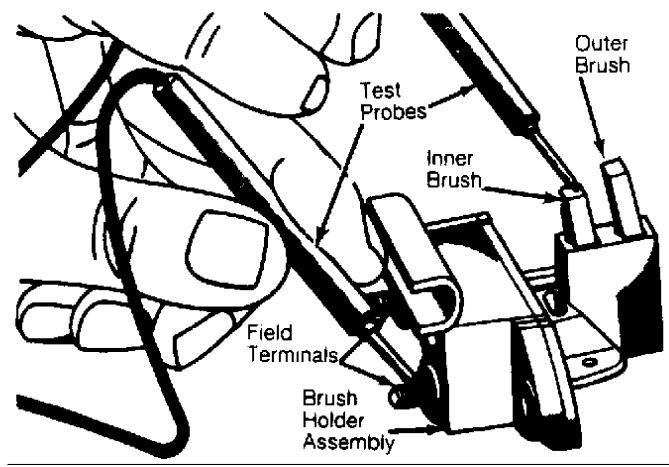
Fig. 18: Testing Inner & Outer Brush Circuit Courtesy of Chrysler Motors.
