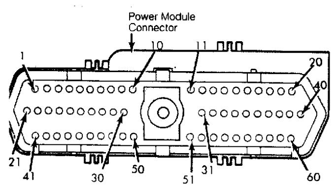
Fig. 8: Power Module 60-Way Connector Courtesy of Chrysler Motors.
