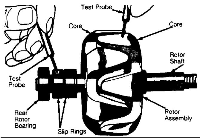
Fig. 12: Testing Rotor Coil for Ground Courtesy of Chrysler Motors.
