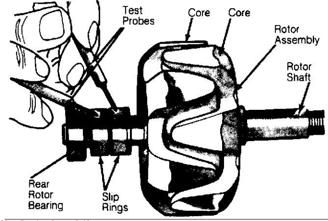
Fig. 11: Testing Rotor Coils Courtesy of Chrysler Motors.
