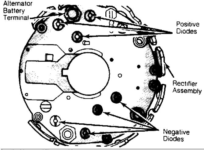
Fig. 15: Checking Rectifier Assembly Courtesy of Chrysler Motors.
