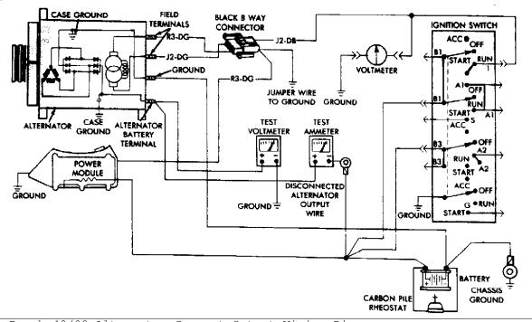
Fig. 4: Bosch 40/90 Alternator Current Output Wiring Diagram Courtesy of Chrysler Motors.
