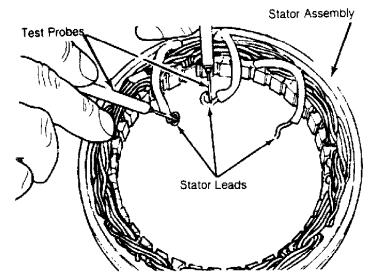
Fig. 14: Testing Stator Coil for Open or Ground Courtesy of Chrysler Motors.
