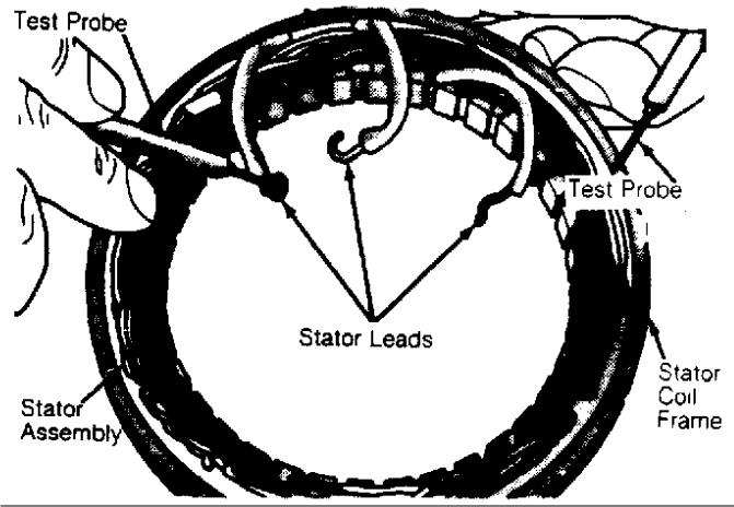
Fig. 13: Testing Stator Coil Ground Courtesy of Chrysler Motors.
