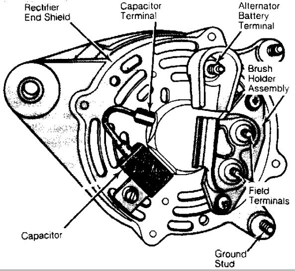
Fig. 1: Rear View of Bosch 40/90 Alternator Courtesy of Chrysler Motors.
