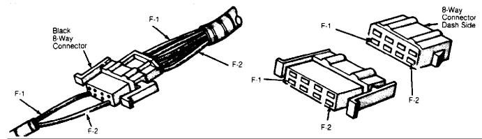
Fig. 6: Identifying F-1 and F-2 Connectors Courtesy of Chrysler Motors.
